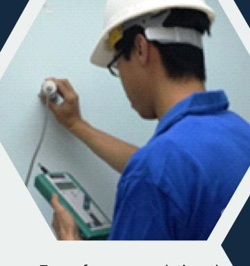
To perform a correlation, the user will input the distance between the two sensors, and the pipe material (if known) into the base unit. Each sensor records the sound and transmits this data to a base unit, which measures the time difference between the leak noise signals arriving at each sensor. From this data, the base unit can calculate the precise location of the leak.
