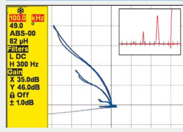
In the case of non-destructive testing (NDT), these are displayed on an eddy current flaw detector as a distinct change in signal. The main advantages of eddy current inspection include:
