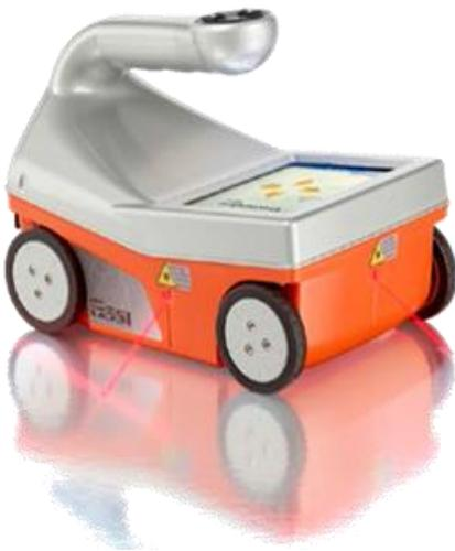
Using the Structurescan radar hand-held system which locates rebar, conduits and post-tension cables in concrete at depths of up to (40 cm), when coring and opening up concrete, will give extra confidence in the conditions immediately under the area to be cored or exposed.
