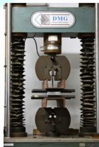
**Flexural testing of tiles**
