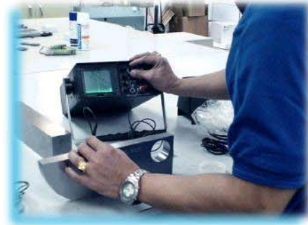
Ultrasonic test equipment being calibrated
