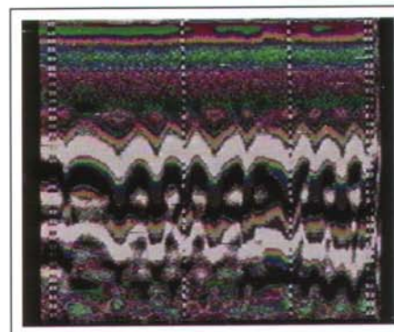
Digitized Radar Signal showing reinforcement details
