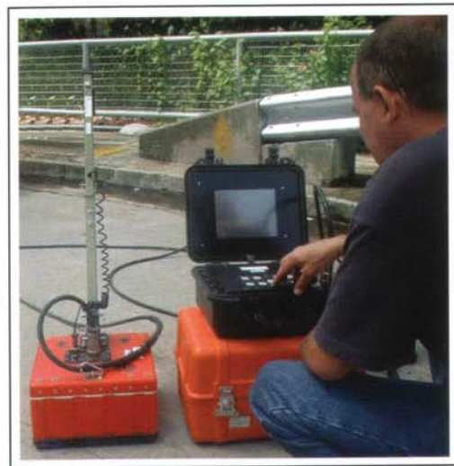
Ground Investigation by Radar
